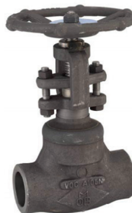
ROBINET SOUPAPE 800LBS A105 A182F6 PASSAGE INTEGRAL SW CHAPEAU SOUDÉ FULL STELLITE TRIMS
